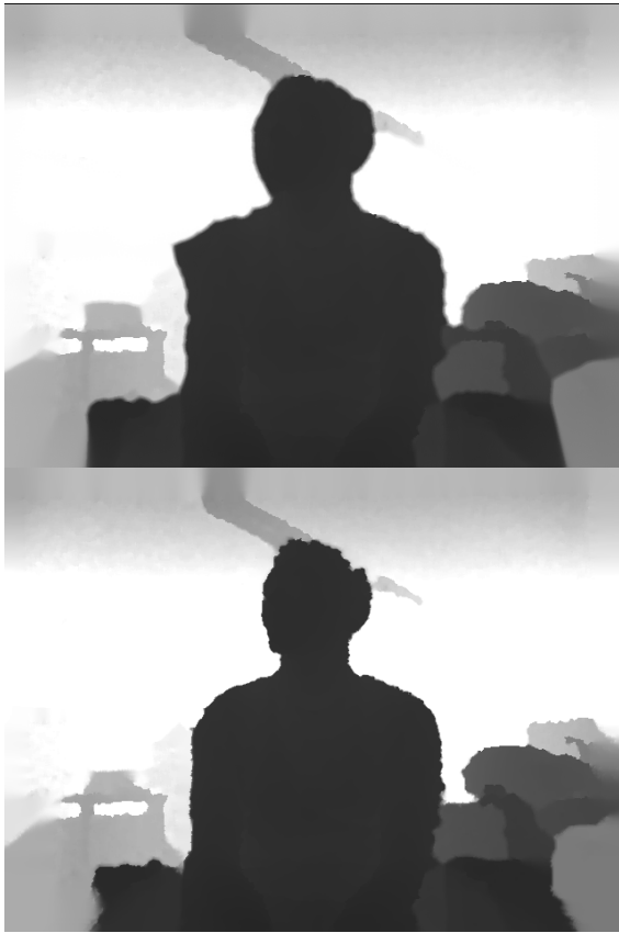
Figure 3. Naive Telea inpainting method (top) compared to our method (bottom).
