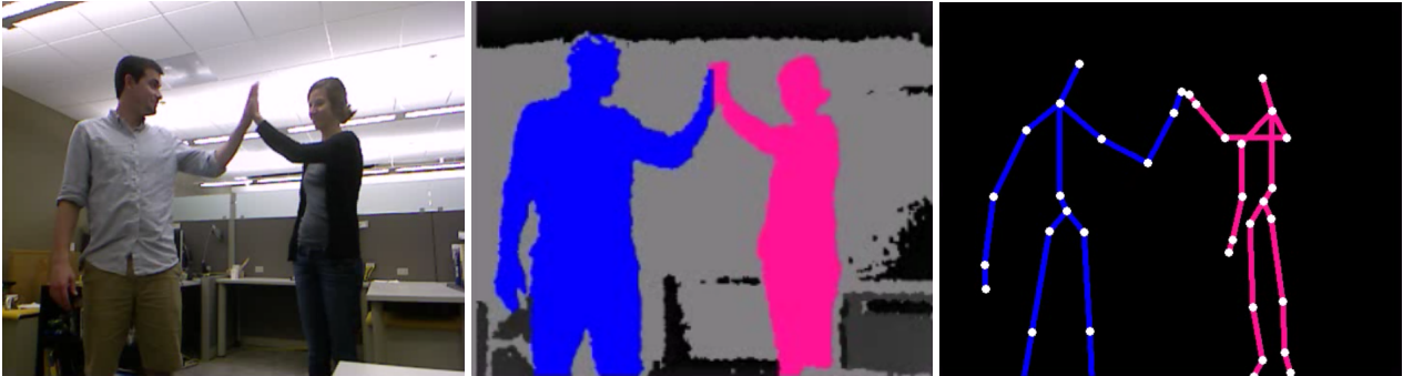
Figure 1. (a) the input RGB image, (b) the depth map overlaid with detected player genders, (c) the skeletal tracking with detected player genders
